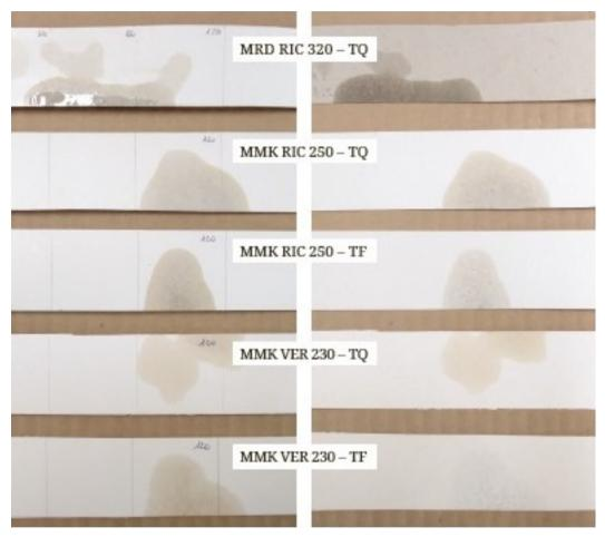
Figure 9 Level of oil absorption in critical temperature conditions (120°C) after 120 minutes. Comparison between uncoated (TQ) and fluorinated paperboard (TF)
