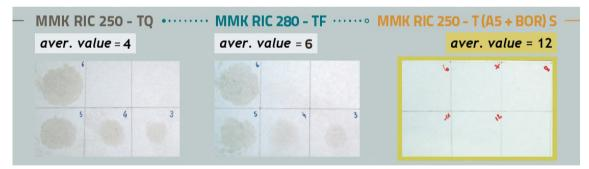
Figure 8 Comparison between the level of oil absorption (Kit Test - TAPPI 559) of uncoated paperboard (sx), fluorinated paperboard (c) and natural-based coatings (dx) on recycled fibre based materials
