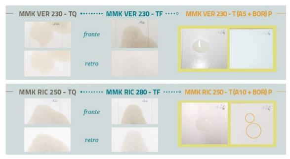
Figure 10 Level of oil absorption in critical temperature conditions  $(120^{\circ}C)$  after 120 minutes. Comparison between uncoated paperboard (sx), fluorinated paperboard (c) and natural-based coatings (dx) on virgin (VER) or recycled (RIC) fibre based materials
