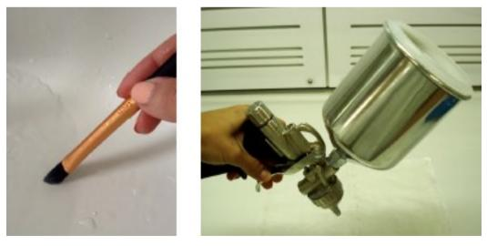
Figure 6 Brushing and spray coating deposition
